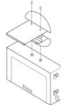
Figure 12: Orienting and Installing the Radio Unit
